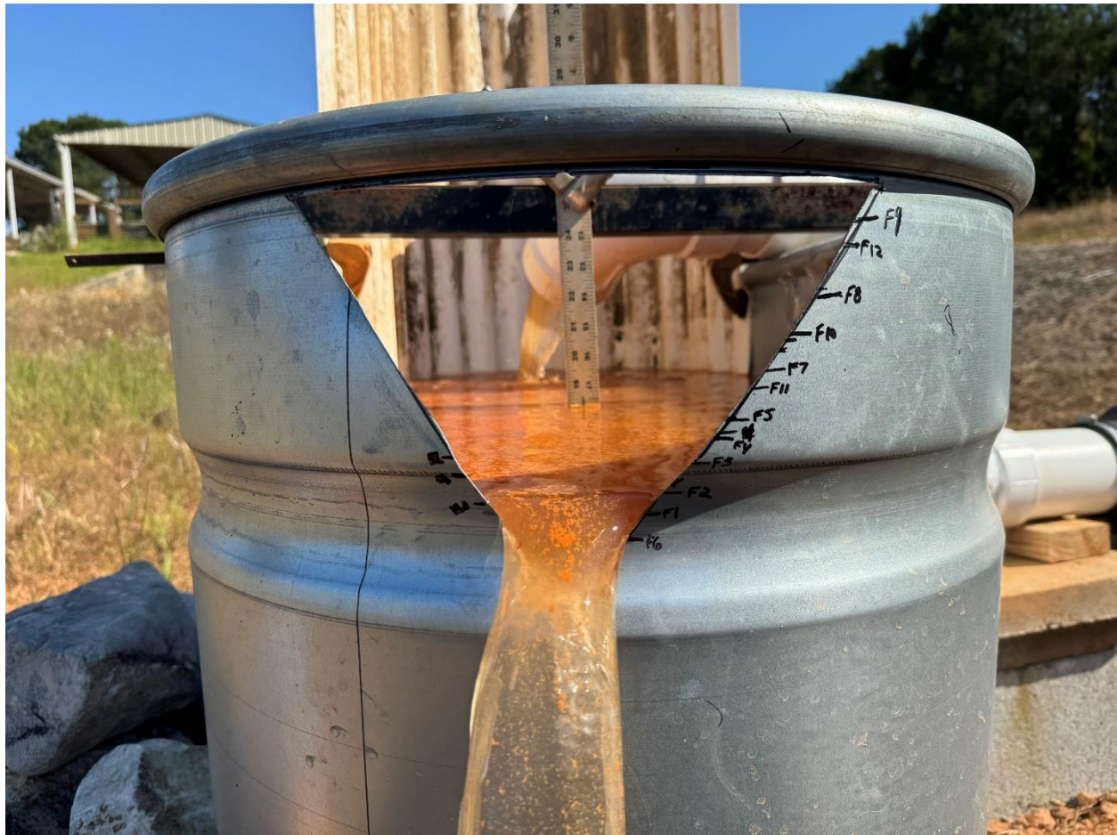
Figure 5.9 Weir Box for Prototype D Evaluations.
