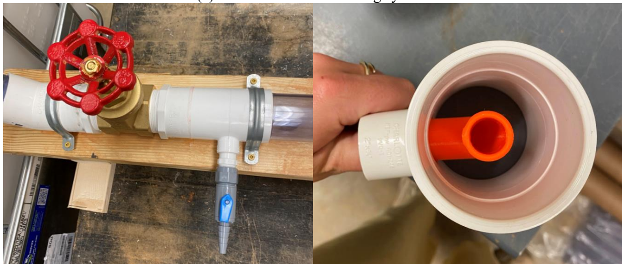
(b) upstream valve and sampling port
