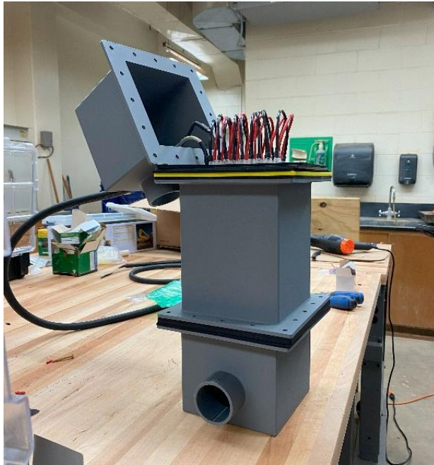
(a) wiring for electrodes
