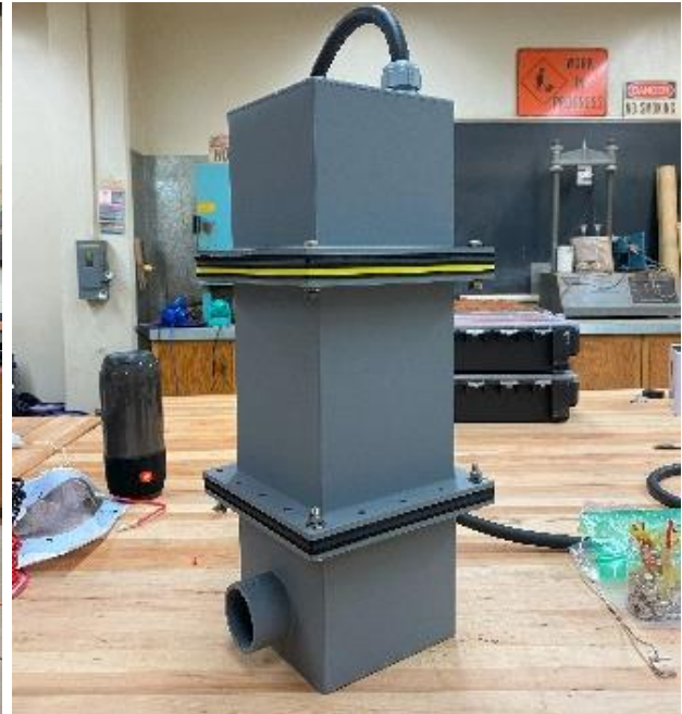
(b) electrode housing
