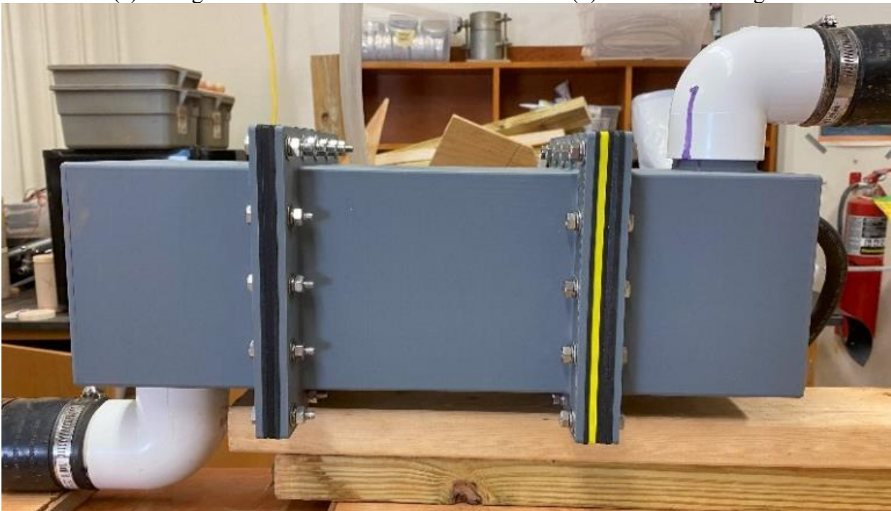
(c) EC installed in bench-scale testing system
