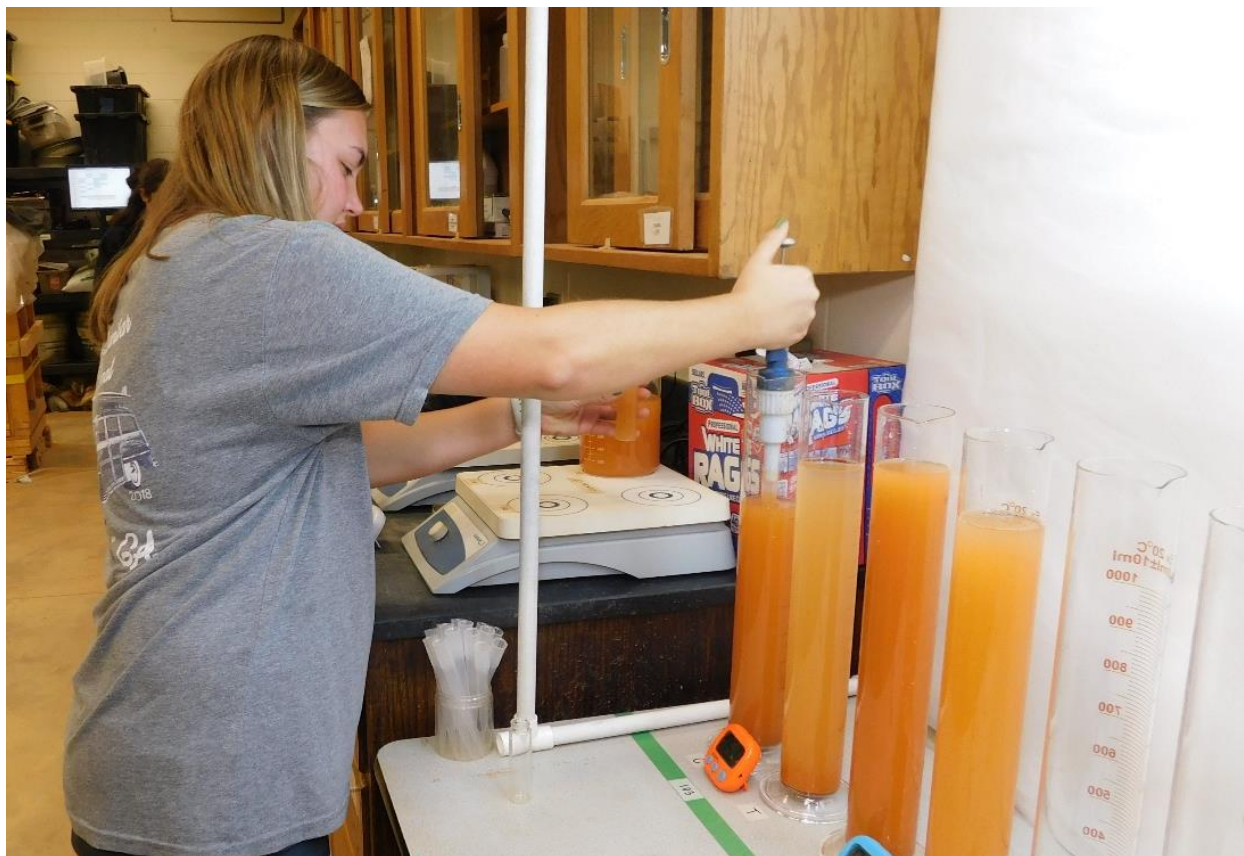
Figure 4.7 Intermediate-Scale Testing: Aliquots Extracted for Turbidity Analysis.
