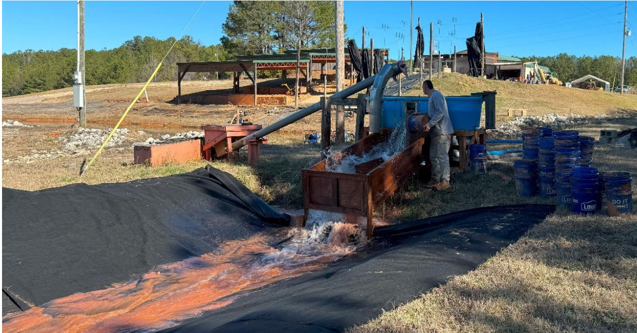
Figure 5.8 Sediment Introduction in Field-Scale Testing.
