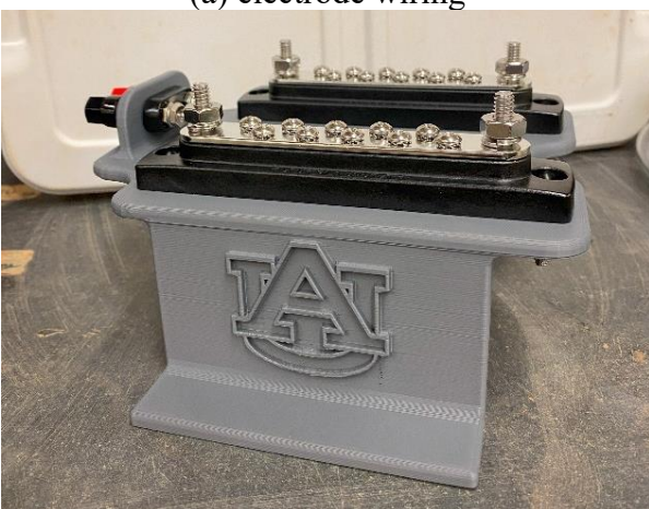
(c) bus bars atop electrode housing
