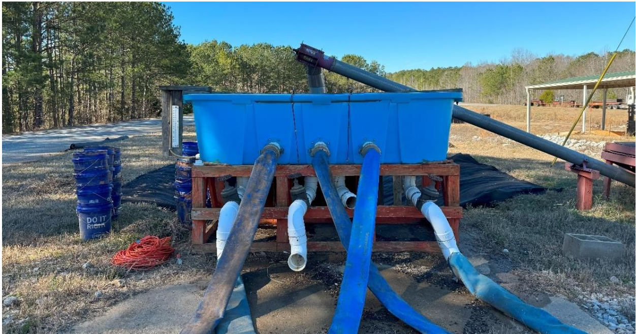
Figure 5.3 Flow Introduction System for Field-Scale Testing.
