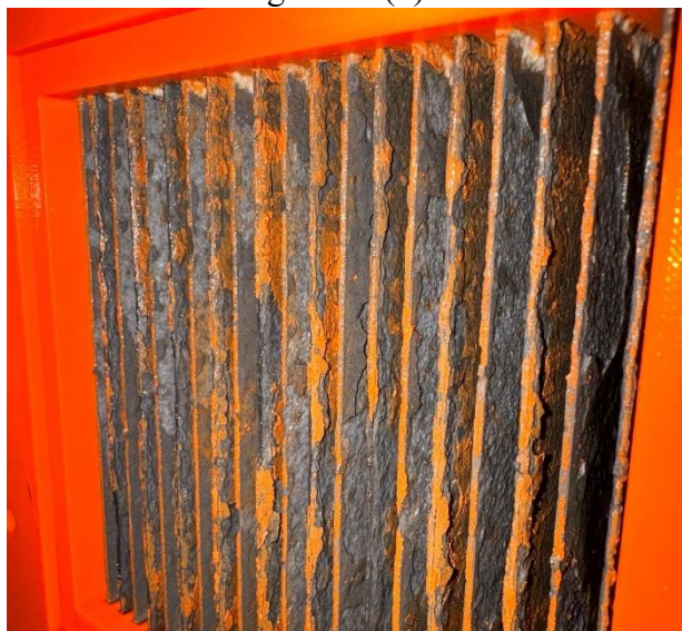
(c) electrodes after rinsing
