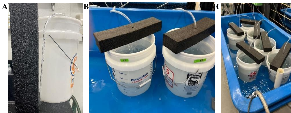
Figure 2.1. Experimental system design. (A) materials used per system, (B) a close-up of two experimental systems, (C) experimental setup including all six systems placed inside a water bath.
