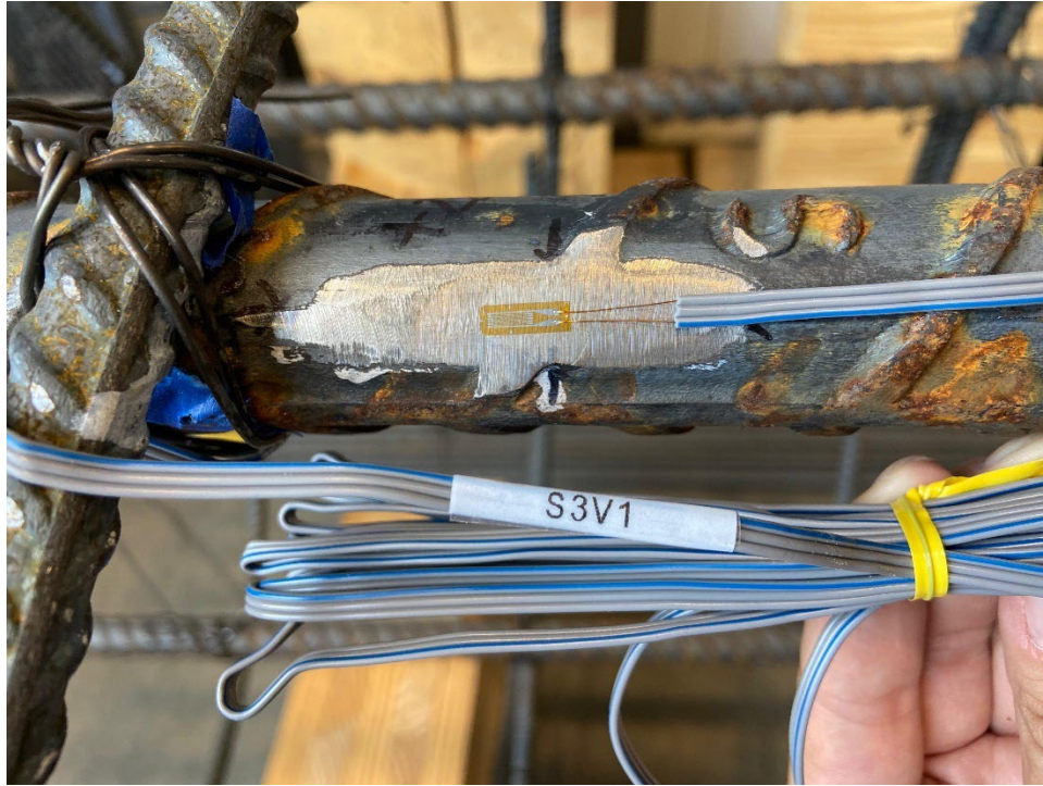
Figure 4-17: Steel strain gauge installed on reinforcing bars
