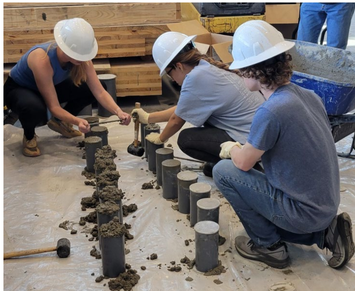
Figure 3-32: Cylinders making process
