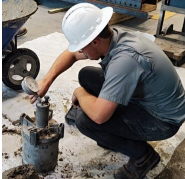
Figure 3-31: Air content test
