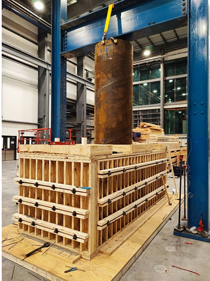
Figure 3-42: Specimen prior to casting
