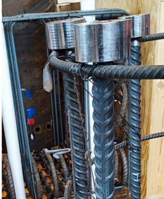
Figure 3-27: Threaded head terminators used for specimen fabrication
