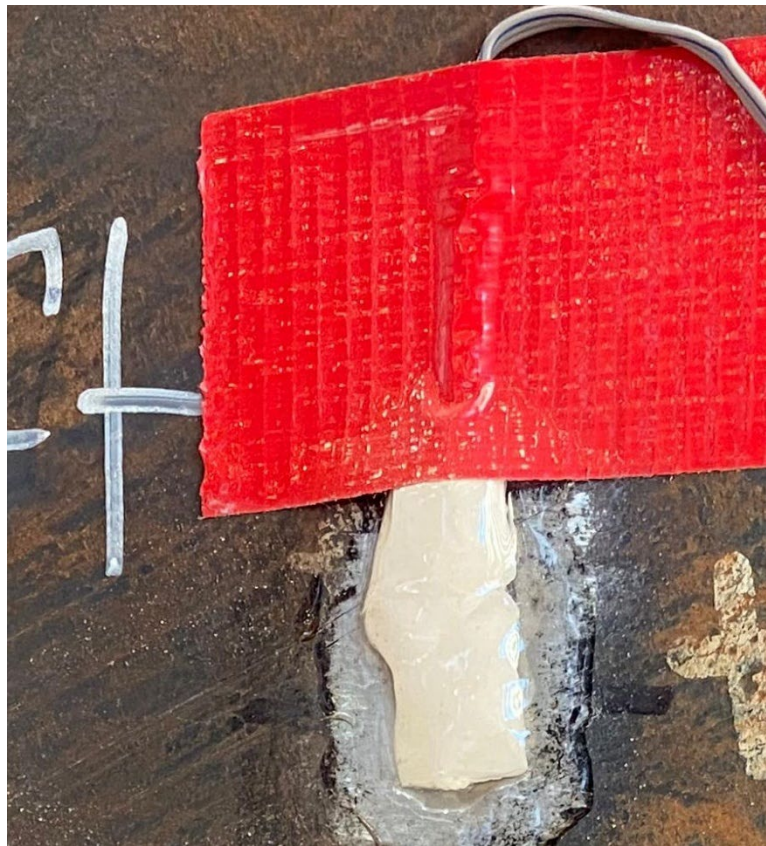
Figure 4-19: Strain gauge after coating
