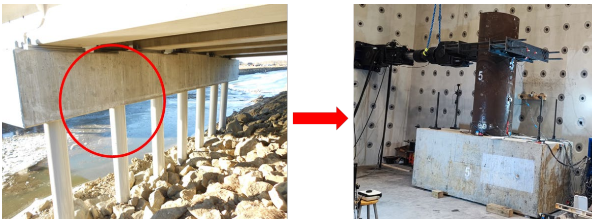
Figure 3-4: Test specimen adapted to laboratory conditions
