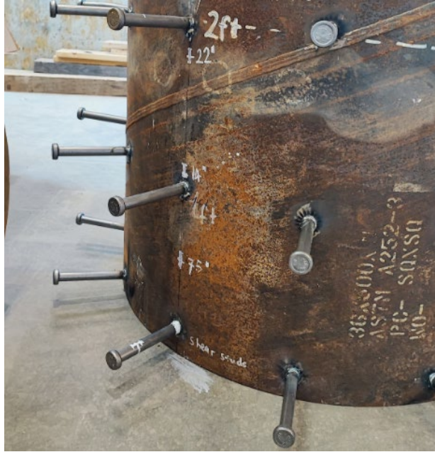
Figure 3-28: Shear studs used for the specimen fabrication
