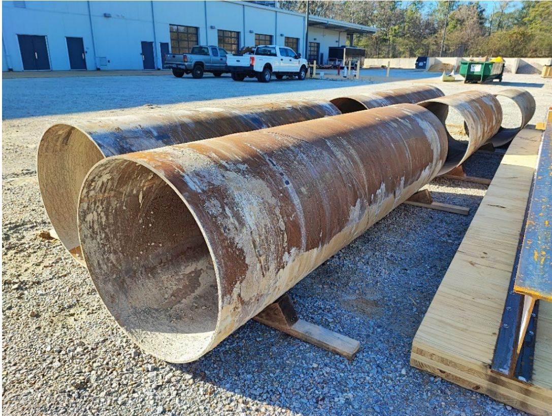
Figure 3-25: Steel pipe piles used for fabrication of specimens
