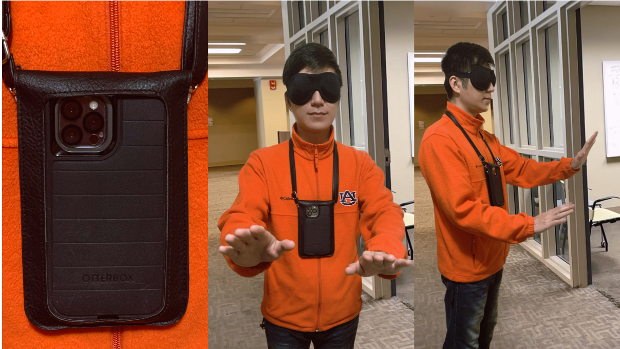
Figure 4.6: Proposed wearable mobility NAAD system by using iPhone 12 Pro Max (right) and sling pouch (left).
