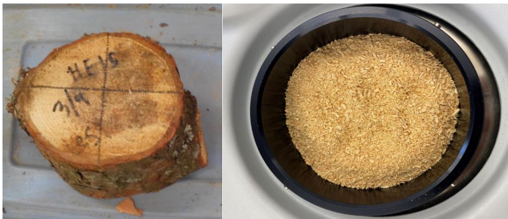
Figure 25: Picture of the Loblolly pine tree disk (on the left) and a ground sample of Loblolly pine species (on the right)
