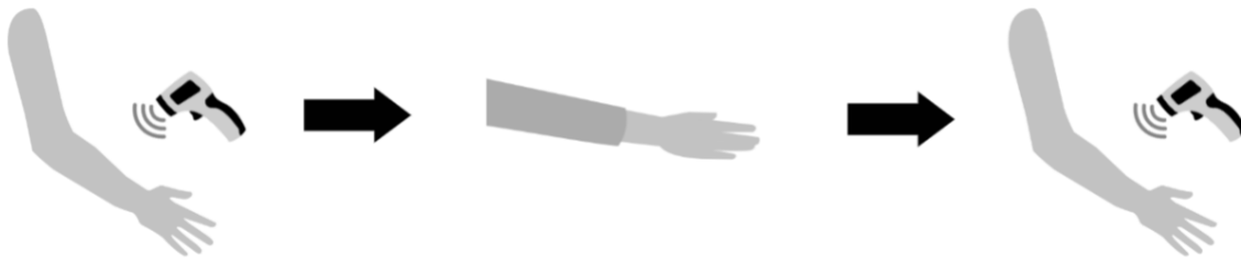
Figure 5 Temperature Difference Test. This figure illustrates the steps in the temperature difference test. An initial temperature is taken before the sleeve is worn and then the temperature is taken again after taking the sleeve off leaving the incubated room.
