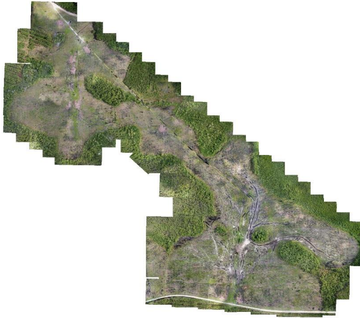
Figure 12. Showing distortion in orthomosaic map around the edges.
