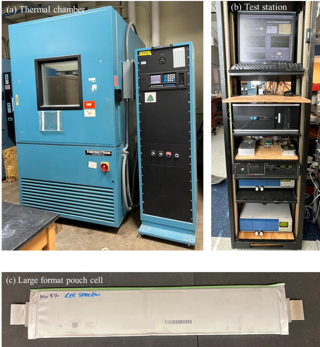
Figure 13. Experiment setup: (a) thermal chamber, (b) overview of a multifunctional test station, (c) a large format pouch type lithium-ion battery.
