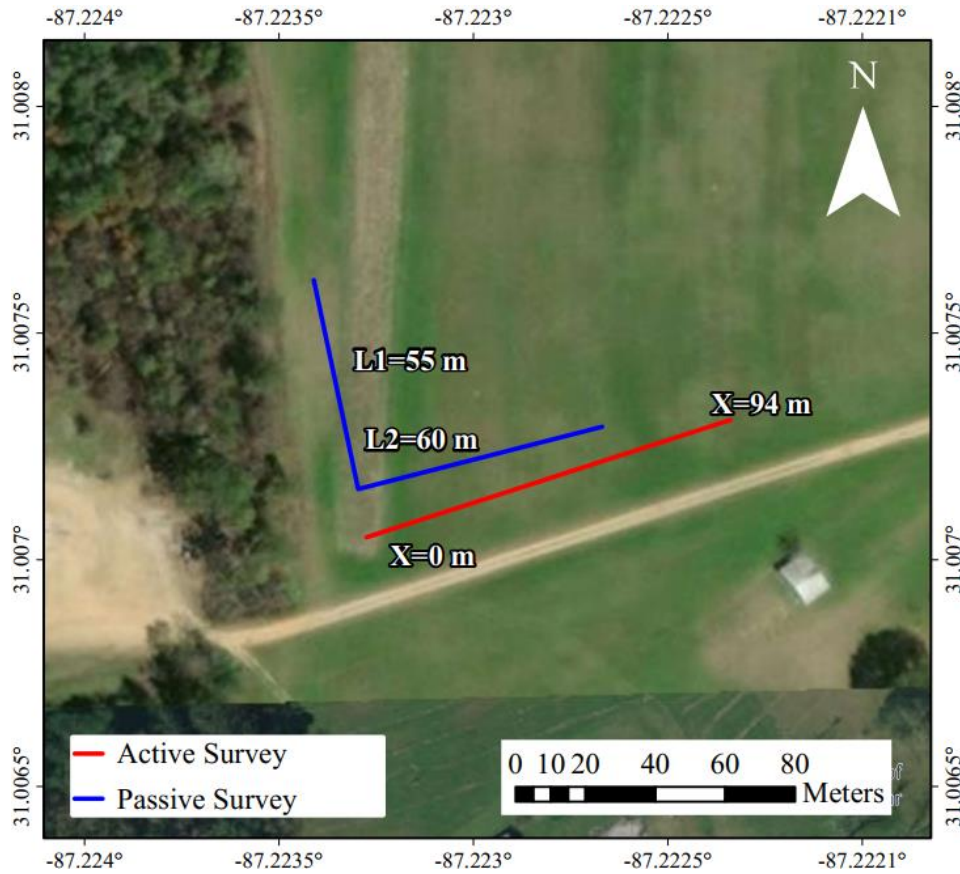
Figure 4-27: Site map with the location of survey line for S2AL seismic station
