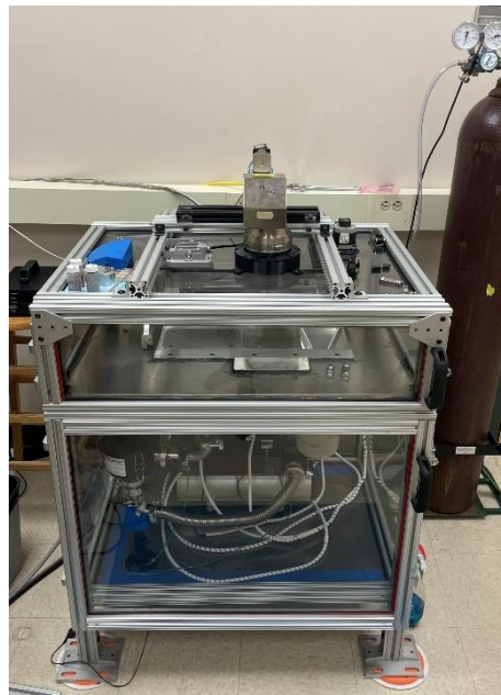
Fig. 3- 3 Custom L-PBF equipped with IPG model YLR-400-AC ytterbium fiber laser.
