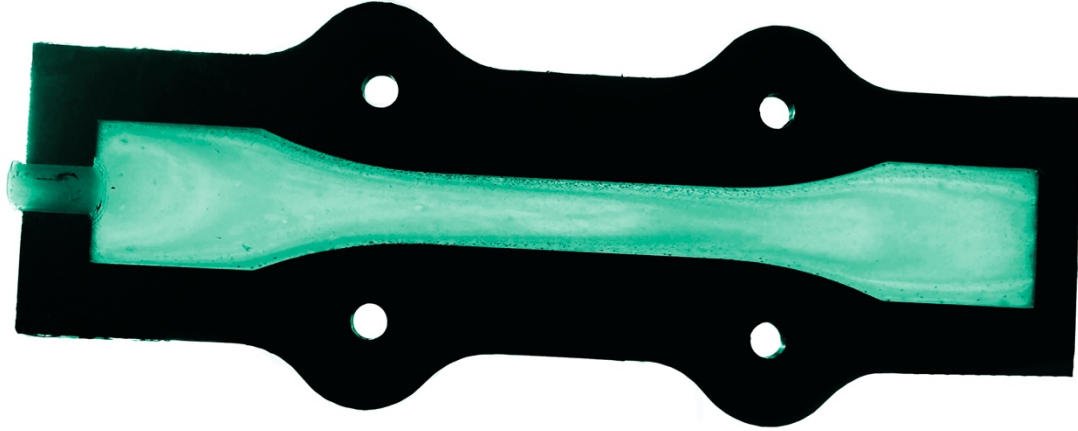
Figure 3.23 CAD Model Representing the Mold and Cured Specimen Removal.
