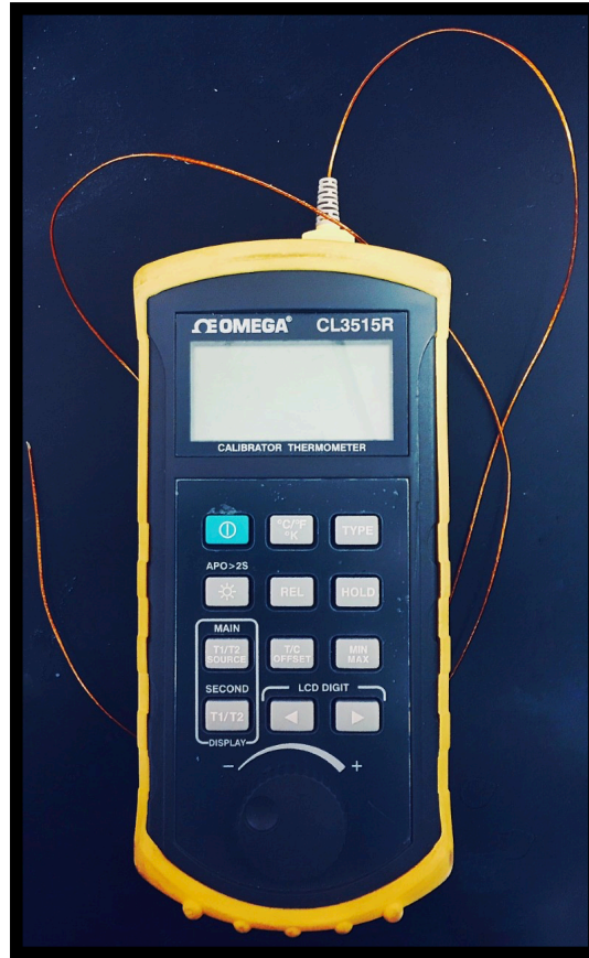
Figure 3.11 Omega Engineering K-type Thermocouple with Uncertainty of +/-2.2 °C
