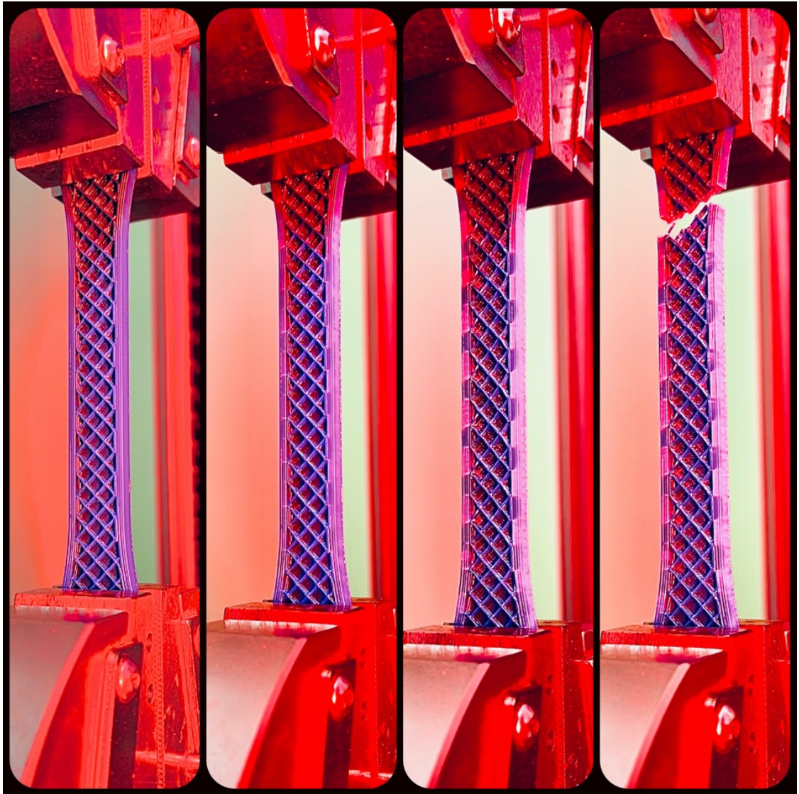
Figure 9.9 Tension Test Performed on Open-faced ABS Specimen with Sparse Infill
