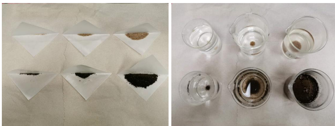
Figure 4.3 The tap water mixed with different masses of sand and topsoil containing organic matters. (a) The mass of 0.05g, 0.5g, and 5g of the sand (on the top) and the topsoil (on the bottom) are shown from the left to the right, respectively; (b) the tap water (200 mL) is mixed with the sand (on the top) and the topsoil (on the bottom) in mixing ratios (w/v) of 0.025%, 0.25%, and 2.5%, respectively.
