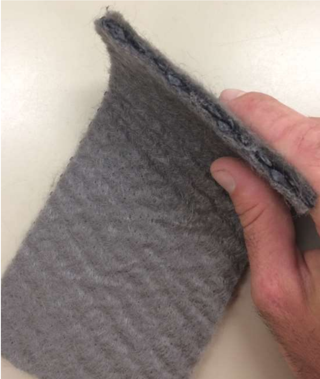
Figure 9: Geonet-nonwoven geotextile composite
