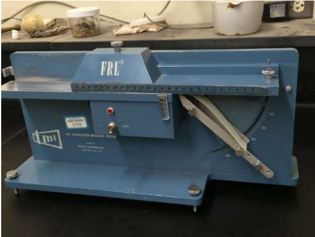
Figure 86: Engineering paper being tested with the FRL Cantilever Bending Tester
