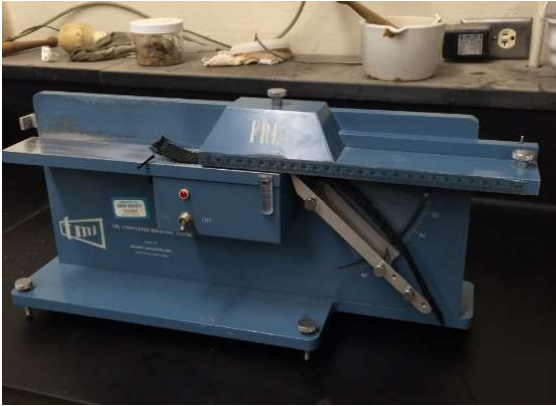
Figure 422: High density polyethylene Cantilever Test 1
