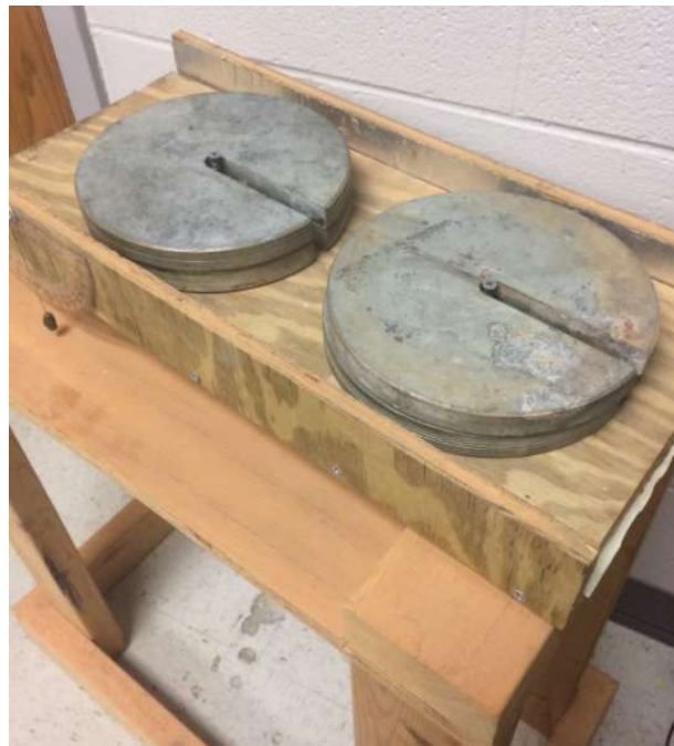
Figure 93: Dead weights placed on top plate, held in place with screws
