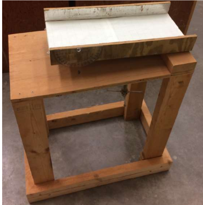
Figure 90: Paper taped to bottom plate of tilt table
