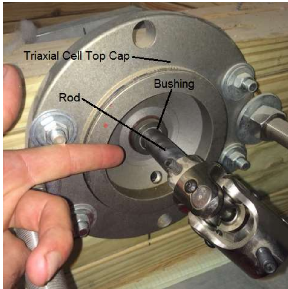
Figure 55: Triaxial cell top cap, bushing, and rod
