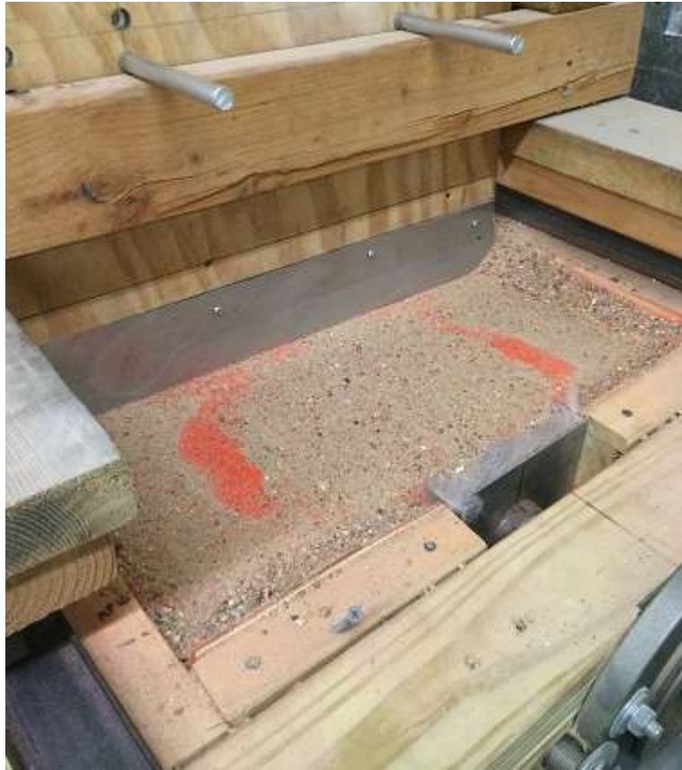
Figure 63: Soil placement device scraping away soil and paint that moved during a test
