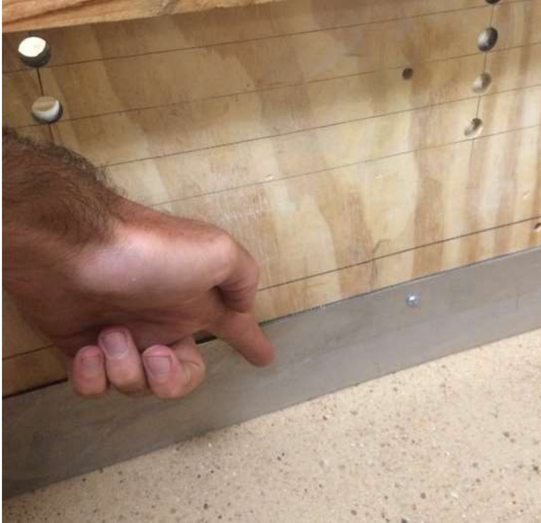
Figure 61: Aluminum straight edge affixed to the bottom of the plate
