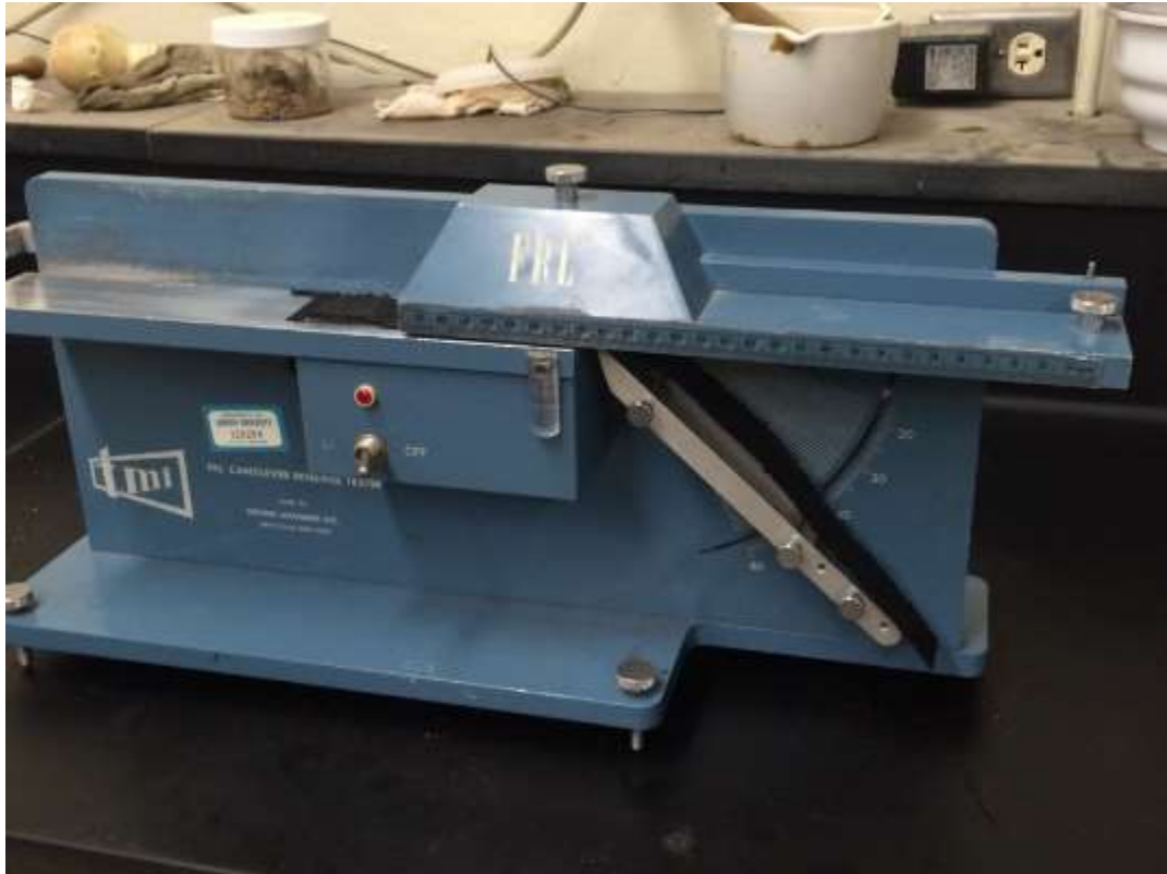
Figure 424: High density polyethylene Cantilever Test 3
