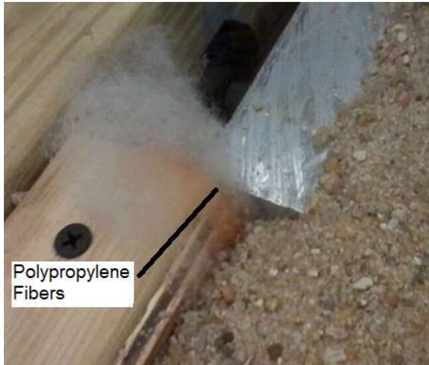
Figure 73: Polypropylene fibers mitigating soil intrusion into the pusher plate-box interface crack during testing.
