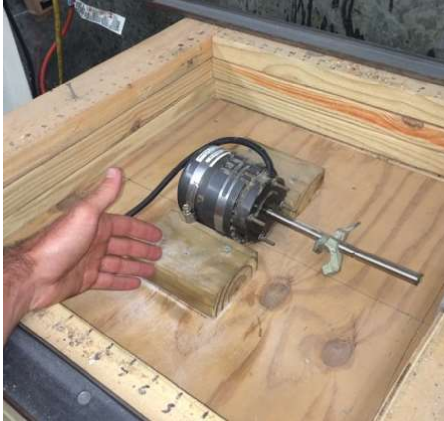
Figure 57: The plate compactor atop a lift of soil, inside the testing box
