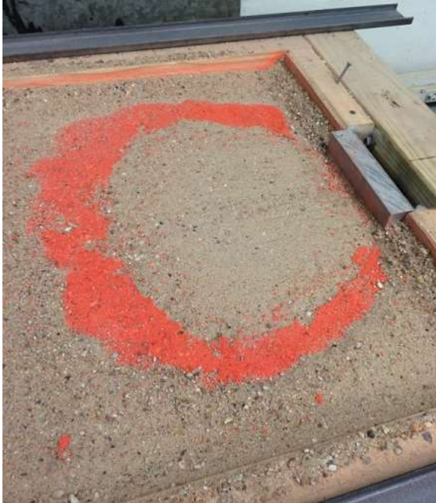
Figure 64: Scraped soil layer revealing failure location
