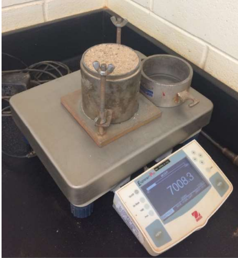
Figure 79: Proctor mold, collar, and compacted sand on balance
