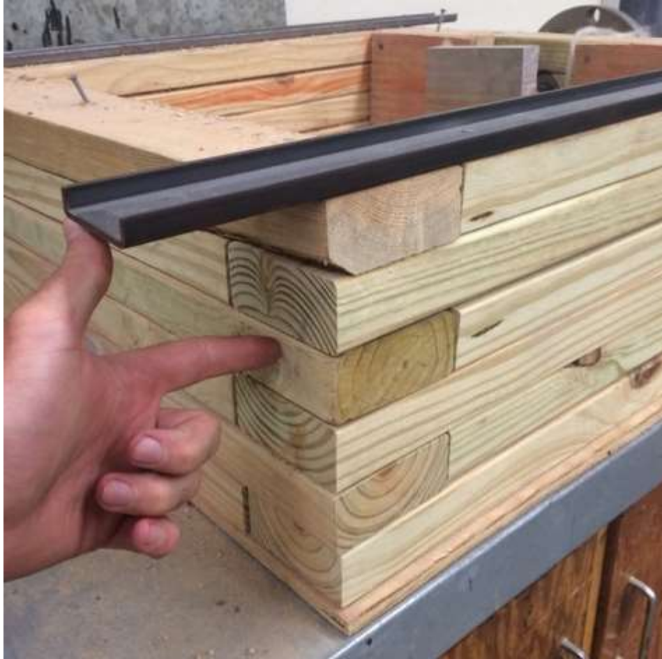
Figure 53: Overlapping corner joint pattern of the box
