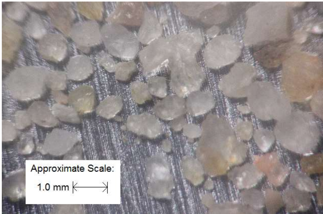
Figure 82: 10X magnified photograph showing various soil particle sizes and shapes
