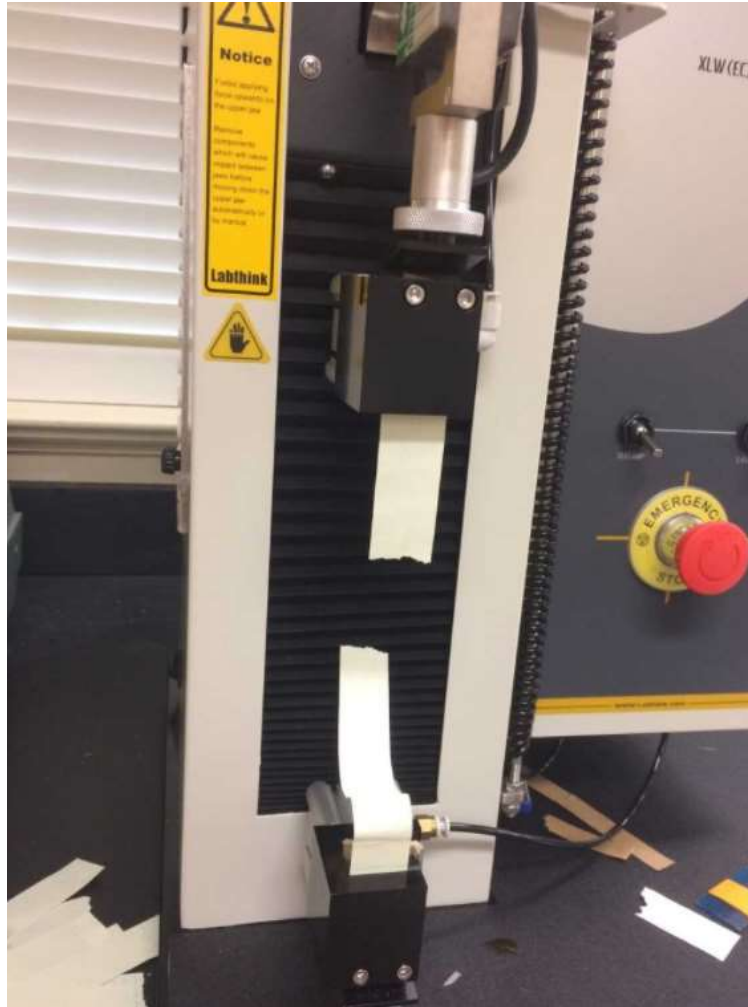
Figure 96: Param XLW(EC) auto tensile tester with ruptured specimen
