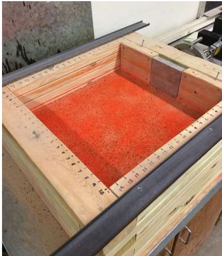
Figure 62: Painted horizontal soil layer
