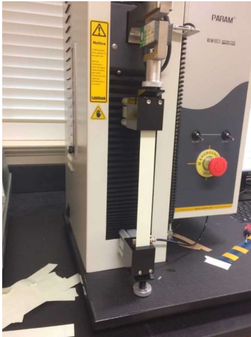
Figure 95: Param XLW(EC) auto tensile tester with paper specimen ready for testing
