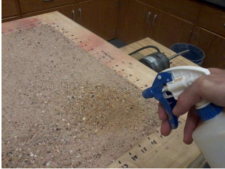
Figure 562: Moistening soil prior to excavation
