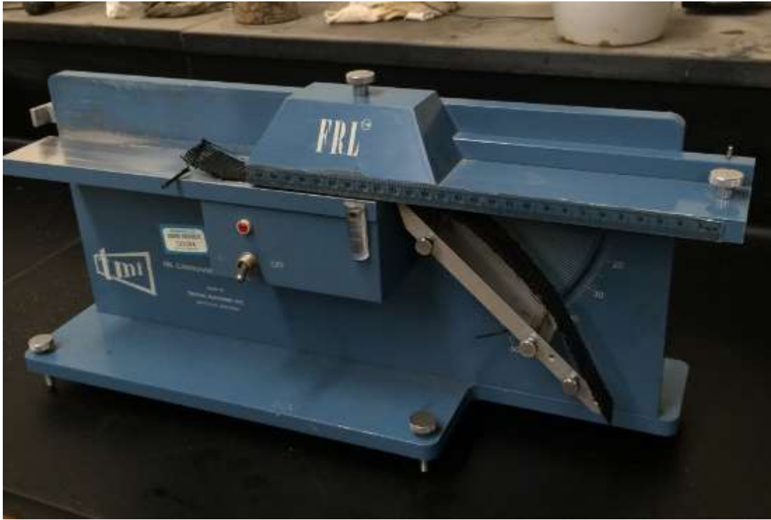
Figure 423: High density polyethylene Cantilever Test 2
