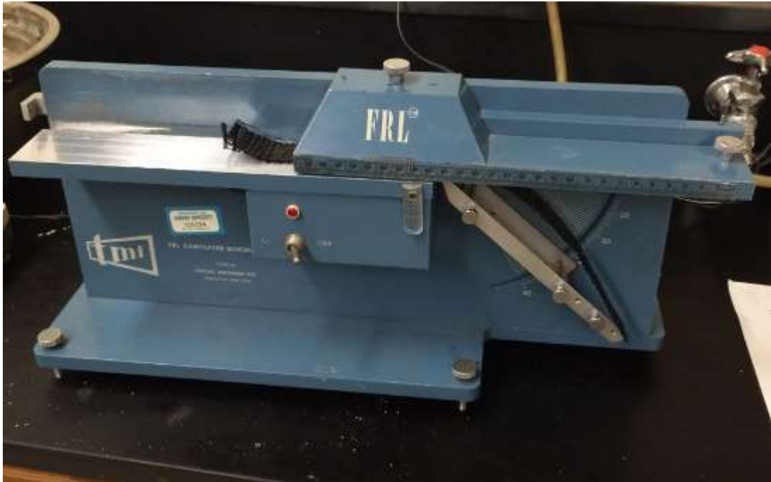
Figure 425: High density polyethylene Cantilever Test 4
