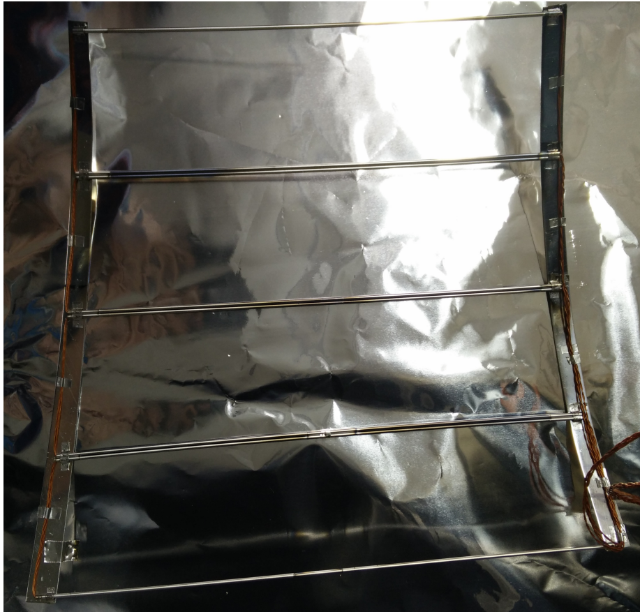
Figure 4.8: One frame of the saddle coils on the bench. Each frame consists of 4 loops.
