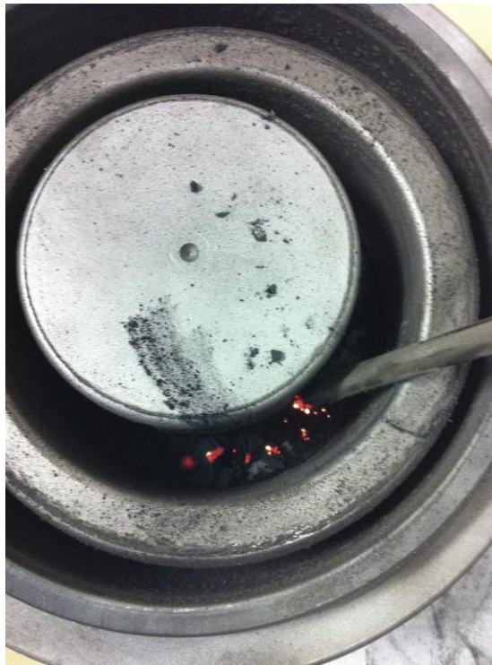
Fig 6-1: Powder burnt during high energy milling process
