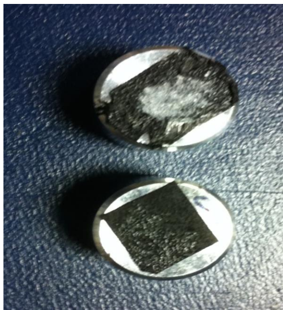
Fig 3-9: Aluminum stub with powders for SEM analysis
