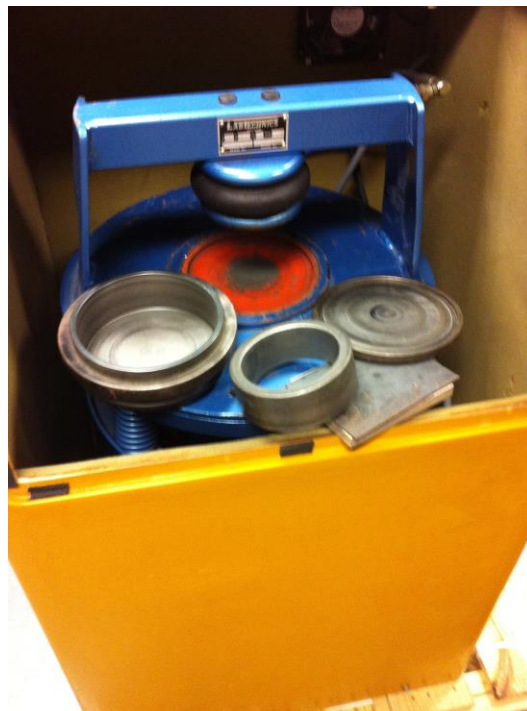
Fig 3-8: Parts of pulverizing mill
