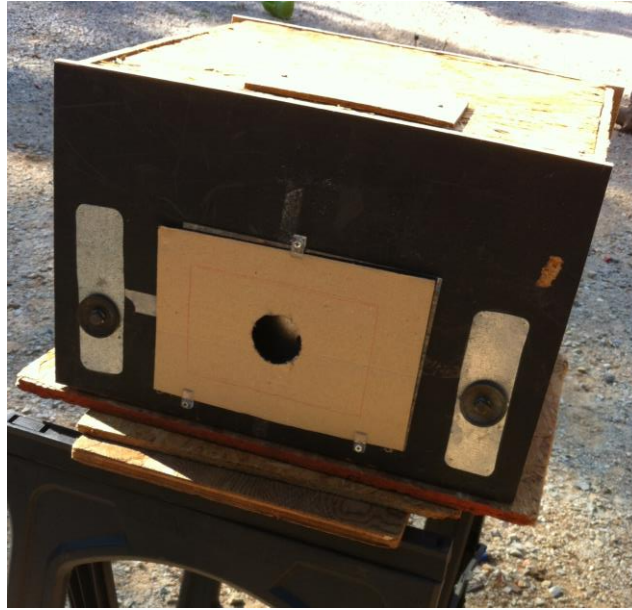
Fig 3-3: Capture box to prevent fly aways
