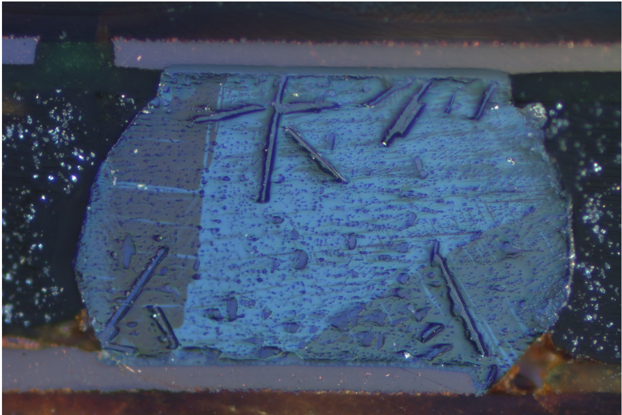
Figure 5.7 Polarized light microscope image of microstructure for a 15mm BGA package solder joint with Paste F including “Beach Ball” structure
