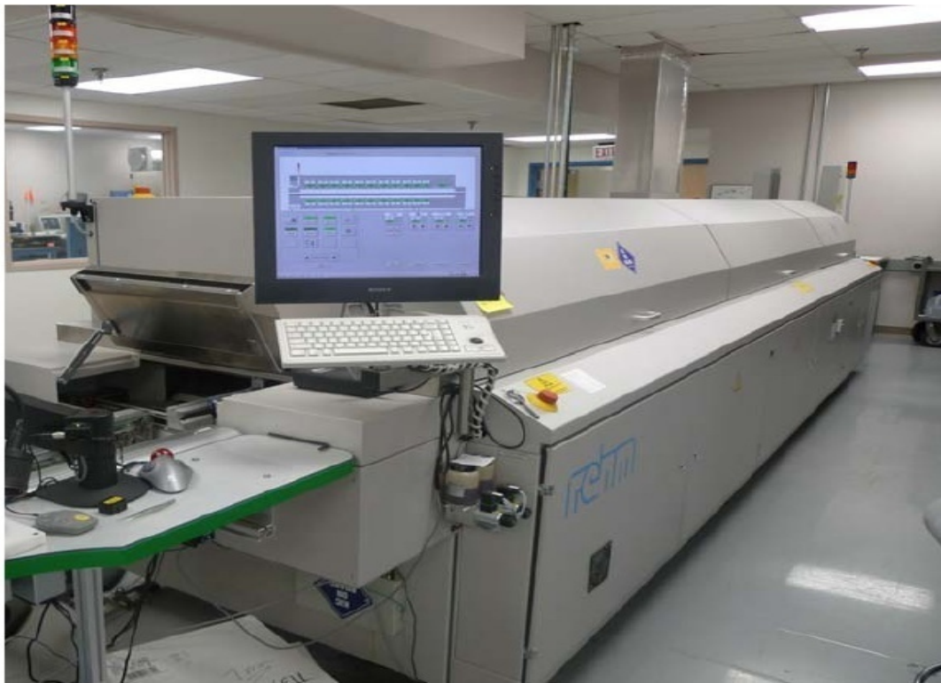
Reflow Oven: Rehm V7
