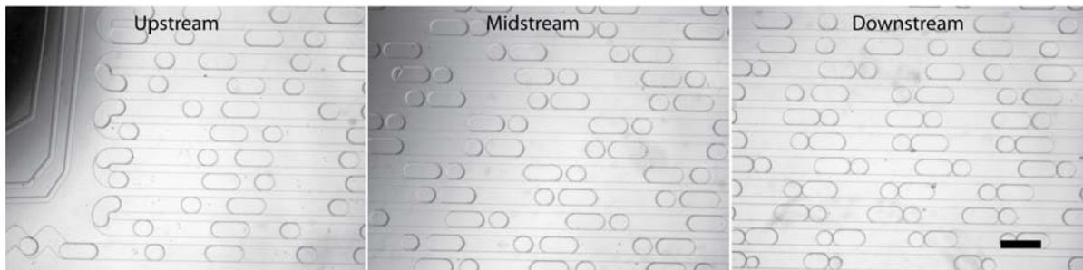
Figure 4.8: Droplets pack up within channels
