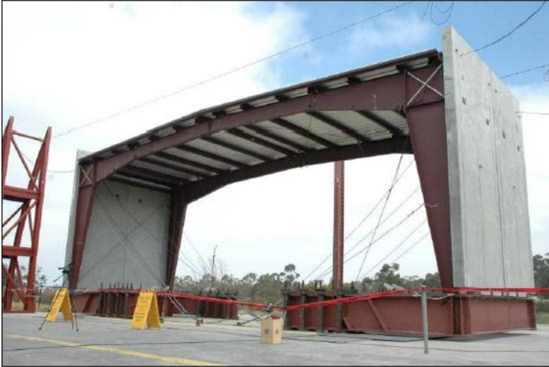
Figure 2.4. Metal Building with Concrete Walls on Shake Table (Smith 2013b)
