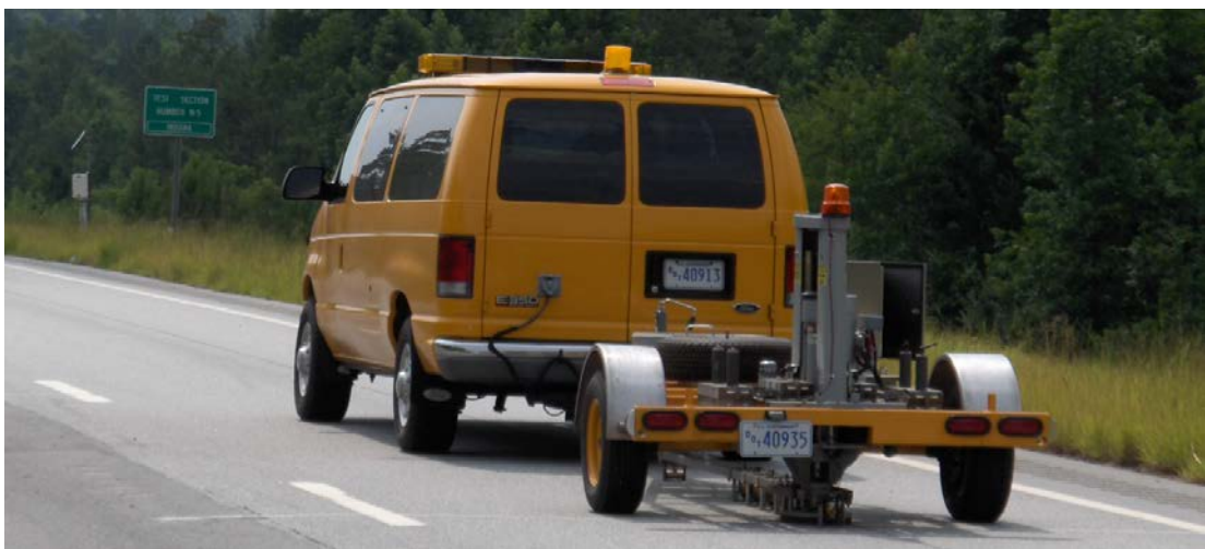
FIGURE 4.5 Falling weight deflectometer testing at the Test Track.
