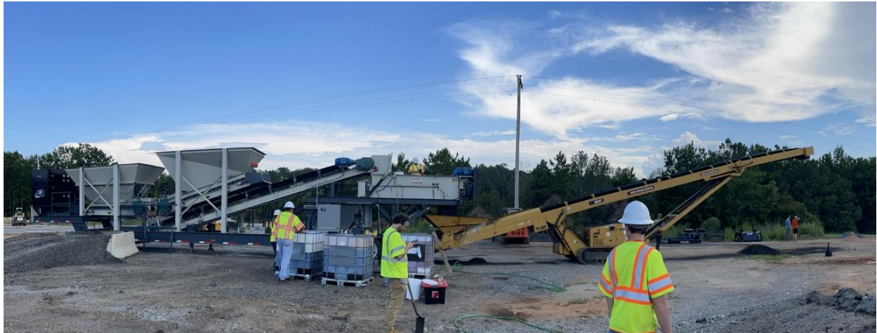
Figure 22. Pugmill Systems Portable Pugmill (Turochy, 2023)
