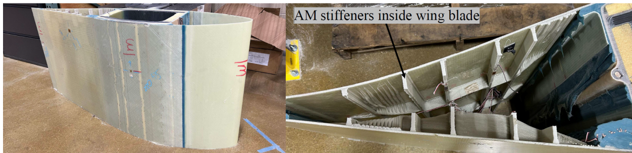
Figure 1.1: Segment of the wind blade tip from the AMERICA program, manufactured via the AM-CM process at ORNL. Large-scale AM stiffeners are incorporated to enhance the blade's fatigue performance under sustained cyclic service loading.
