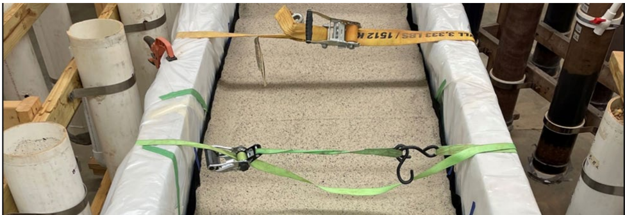
Figure 2.13: Iron-Enhanced Sand Layer
