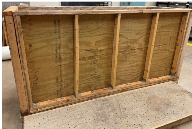
(a) infiltration trench box & false floor
