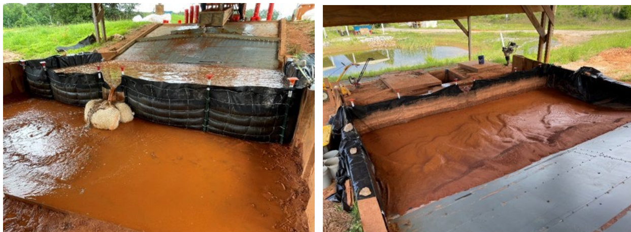
(a) during test (b) post test Figure 3.25: During and Post-Test Photos of Silt Fence
