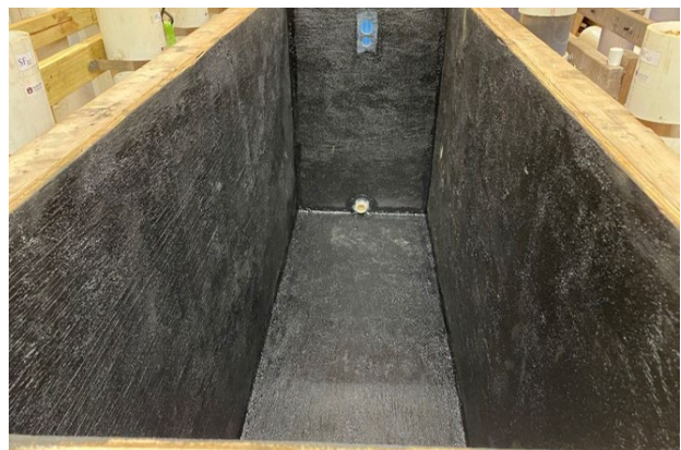
(b) waterproofing layer
