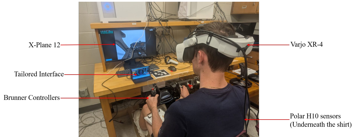
Figure 18 Experiment setup showing the Varjo XR-4, Polar H10 heart-rate sensor, flight controls, simulator displays, and tailored interface display
