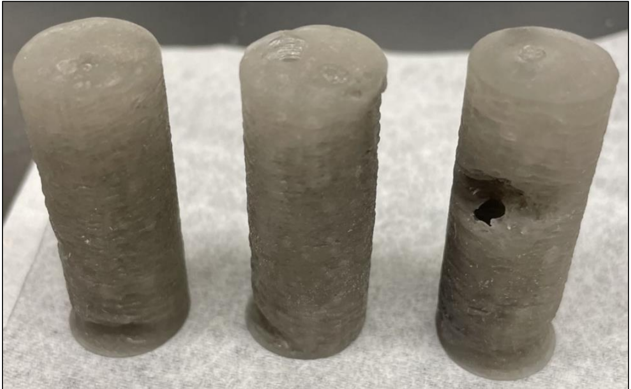
Figure 28. Example failed prints demonstrating substantial air inclusions resulting from mixing speeds of 300 rpm and above.
