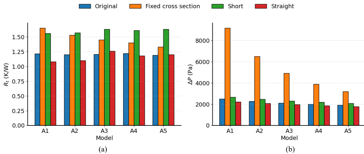
Figure 4.5: Thermo-hydraulic performance of the Group A configurations and their corresponding reference models: (a) thermal resistance and (b) pressure drop.
