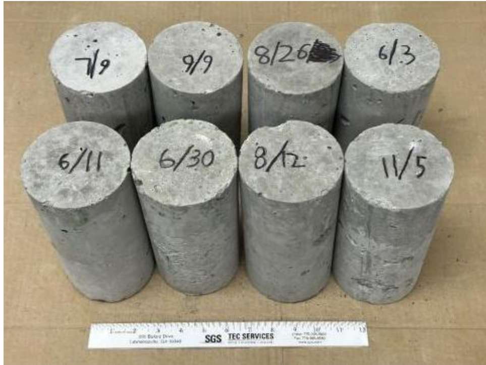
Figure 3-16. Cylinders sent for hardened air-void analysis.
