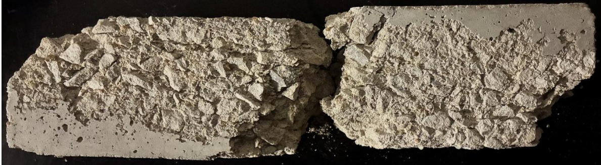
(a) Durability Factor: 4, Mixture ID = 0.45: WR 1
