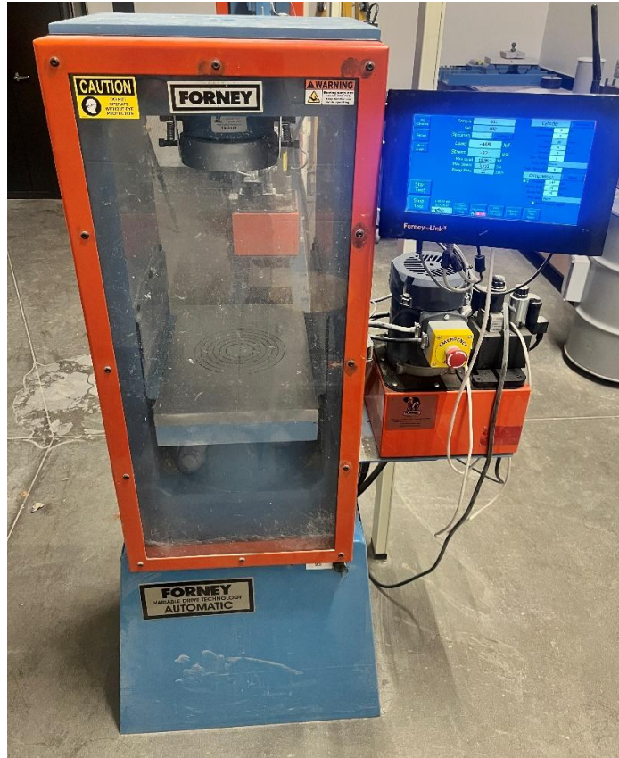
Figure 3-13. Compression test apparatus used in this study.
