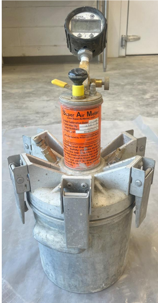
Figure 3-9. Sequential air meter (SAM) made by Humboldt Manufacturing Company.
