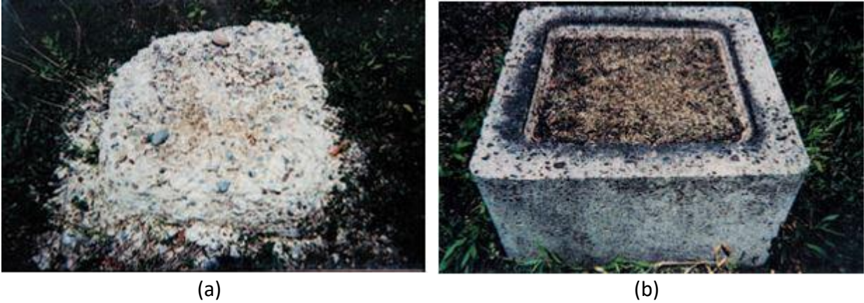
Figure 1-3. Effect of Cycles of Freezing and Thawing on Two Weathering Boxes over the Course of 40 Years. The box on the left (a) is non-air-entrained while the box on the right (b) is air-entrained. (Kosmatka et al. (2002).
