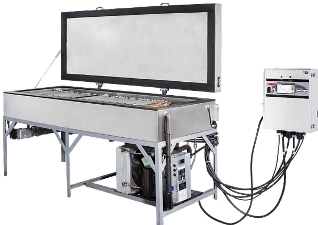
Figure 1-5. Freeze-Thaw Cabinet used for AASHTO T 161 Testing.
