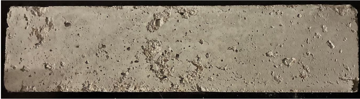
(b) Durability Factor: 33, Mixture ID = 0.45: N+WR 9
