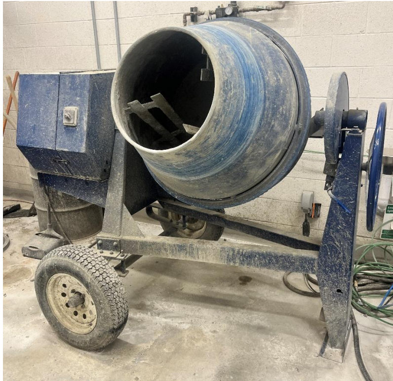
Figure 3-6. Mixer used for batching concrete in this study.
