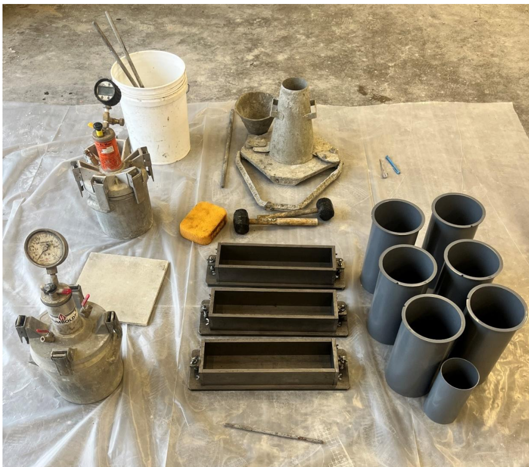
Figure 3-8. Layout for fresh concrete testing and prism and cylinder creation.
