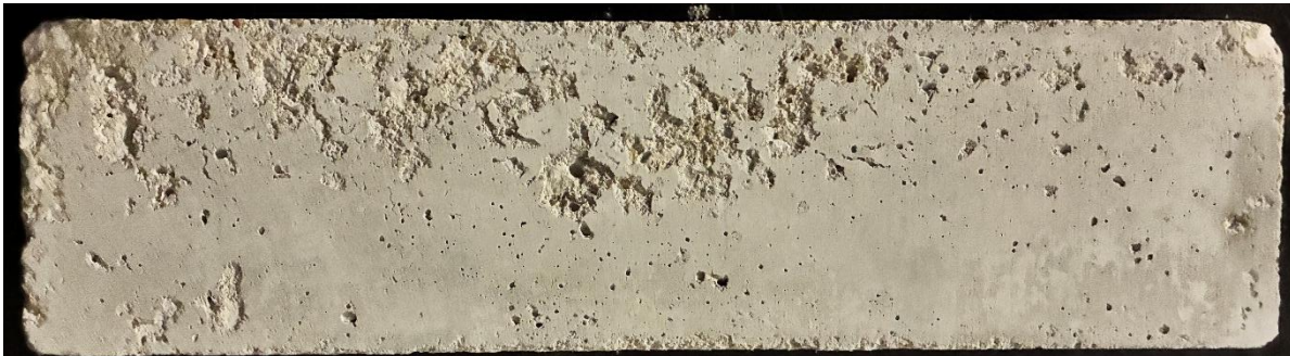
(c) Durability Factor: 74, Mixture ID = 0.50: S+WR 3
