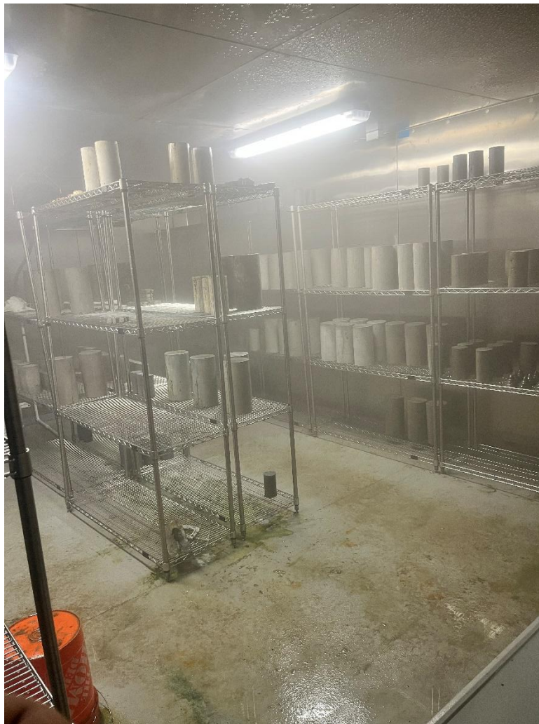
Figure 3-11. Moist room used for curing concrete cylinders.
