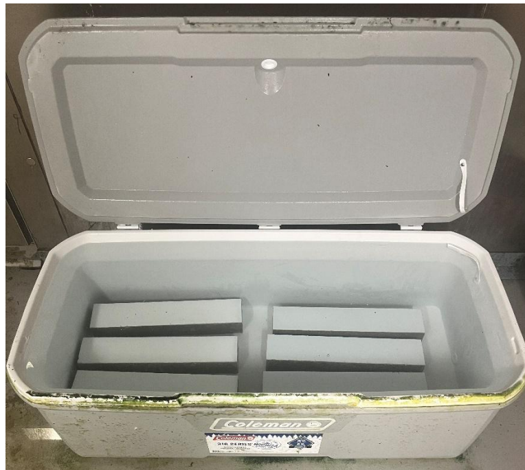
Figure 3-12. Hydrated lime-saturated water bath used to cure freeze-thaw testing prisms.
