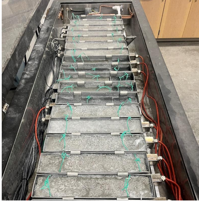
Figure 3-15. Inside chamber of freeze-thaw machine filled with frozen prisms.
