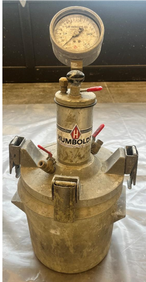
Figure 3-7. Type B pressure meter used in this study.
