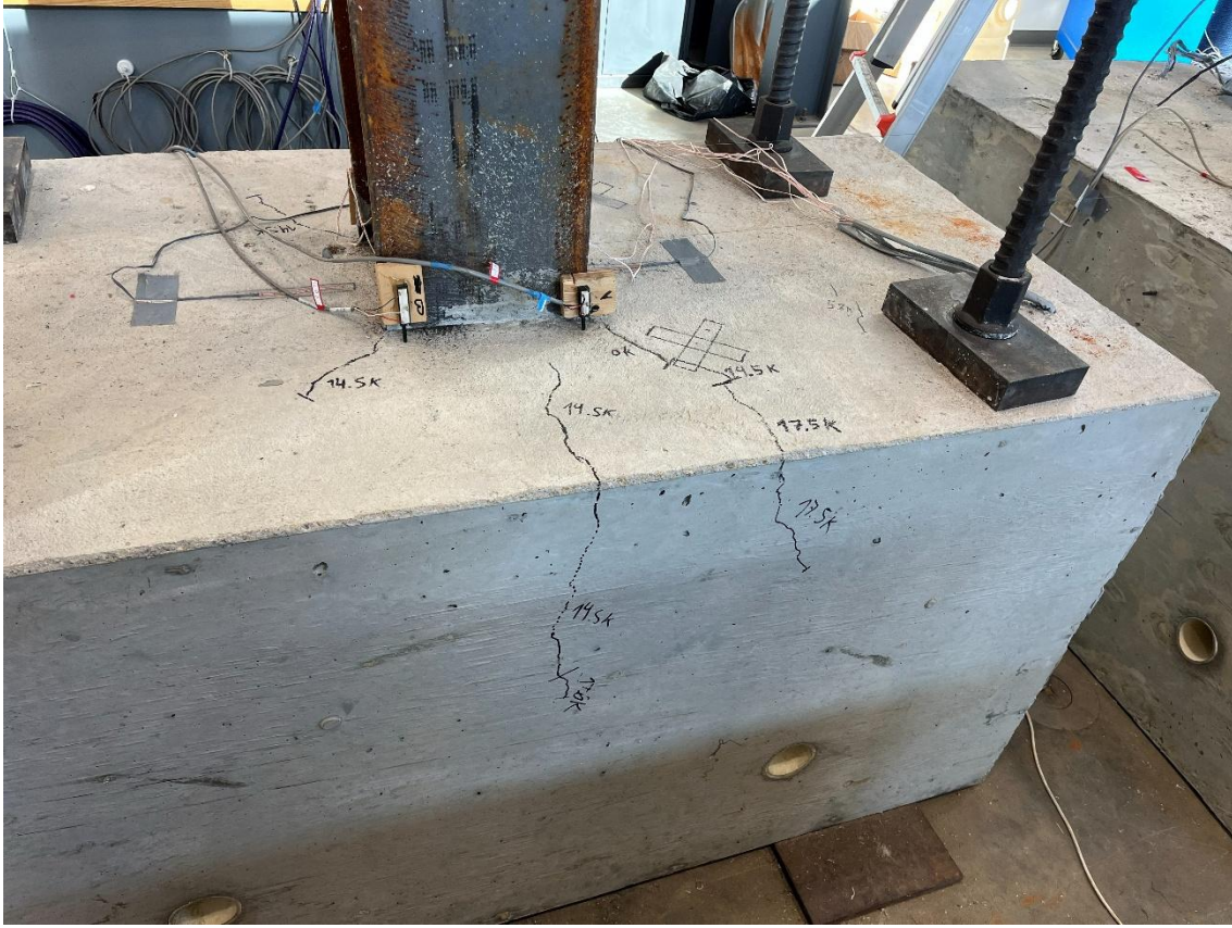
Figure 115. Specimen W-10-10 crack formation after target loads of 14.5 kips and 17.5 kips (applied loads of 14.6 kips and 15.1 kips, respectively) (load direction: from right to left).
