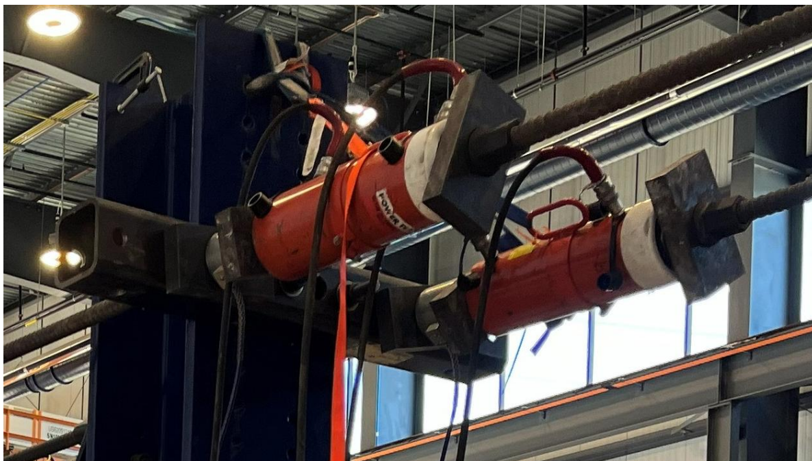
Figure 101. Load cells positioned behind each hydraulic jack during the load test.
