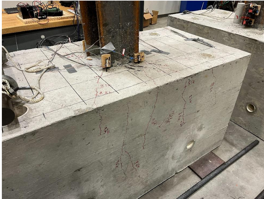
Figure 269. Specimen W-10-7.5 (1 st try) crack formation after target loads of 10.3 kips (applied load of 9.4 kips) (load direction: from right to left).
