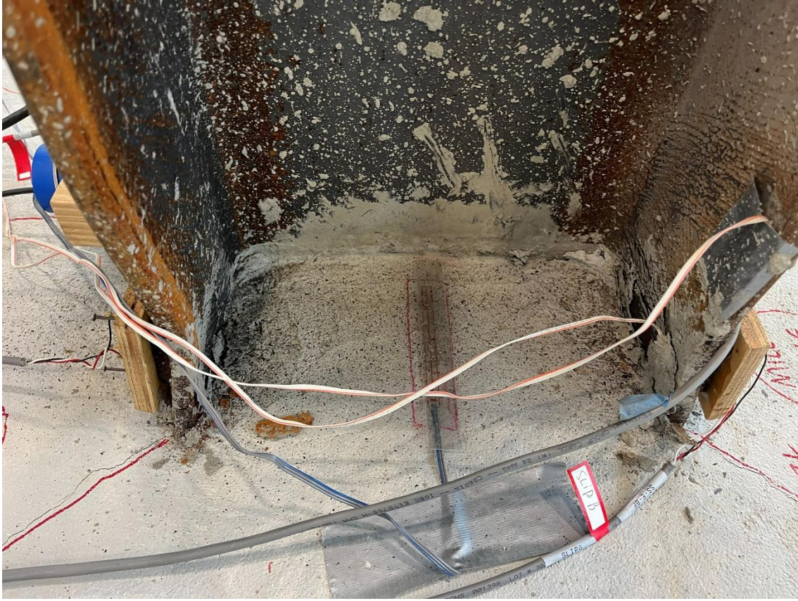
Figure 149. Specimen W-12-12 after final load stage (approx. 23.2 kips). Observed buckling in flanges B and C and mill scale loss.
