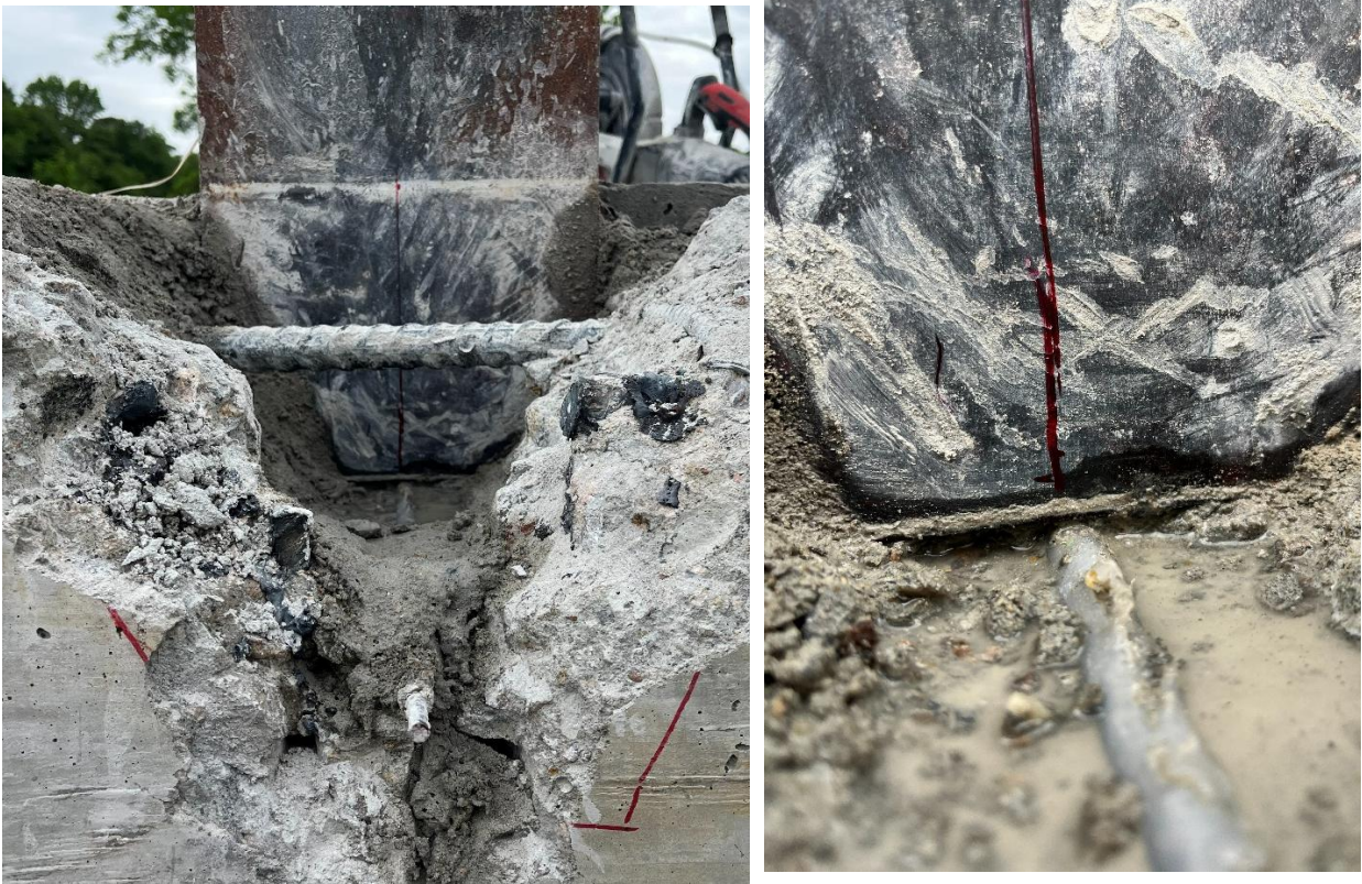
Figure 118. Specimen W-10-10. Demolished specimen showing the final position of the pile head inside the embedded zone.
