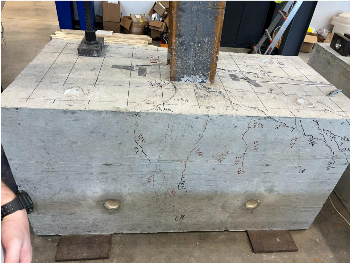
Figure 270. Specimen W-10-7.5 (2 nd try) crack formation after target loads of 13.4 kips (applied load of 8 kips) (load direction: from right to left).
