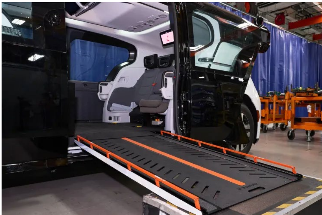
Figure 50. Double-Wide Doors and Ramp (Hawkins, 2023).
