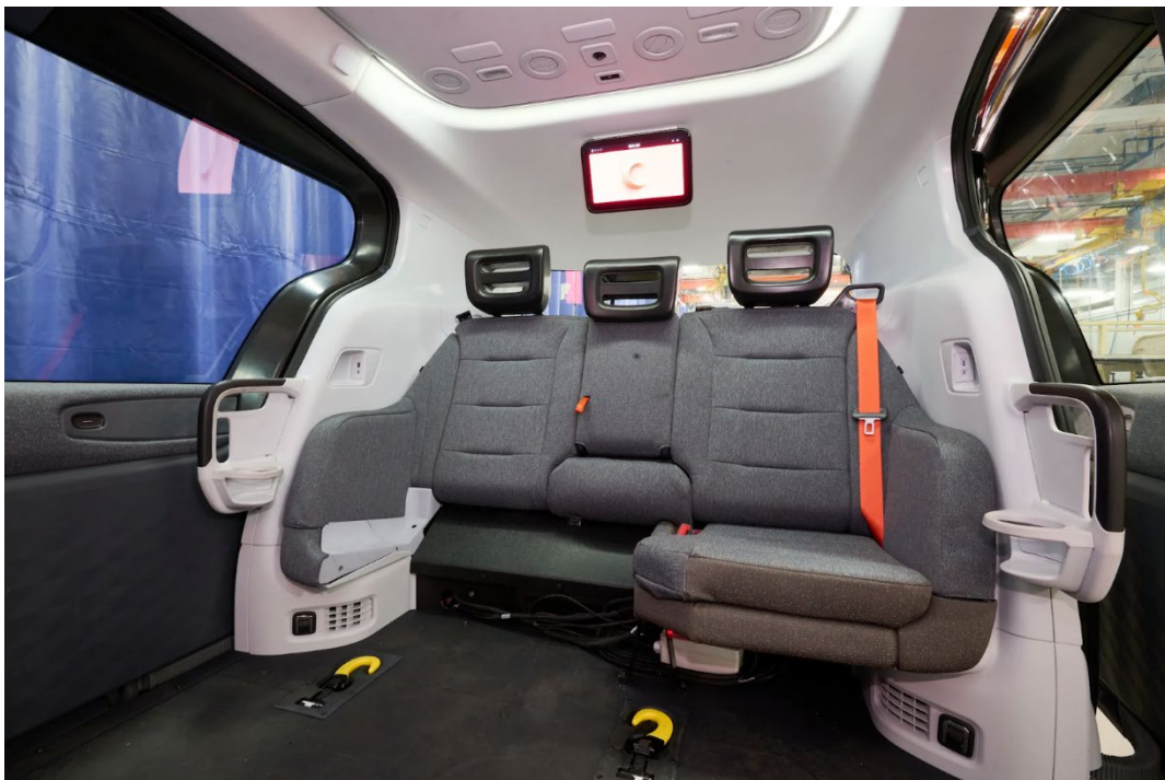
Figure 54. Cruise WAV's Interior Space and Fold-Down Seating Arrangement (Hawkins, 2023).
