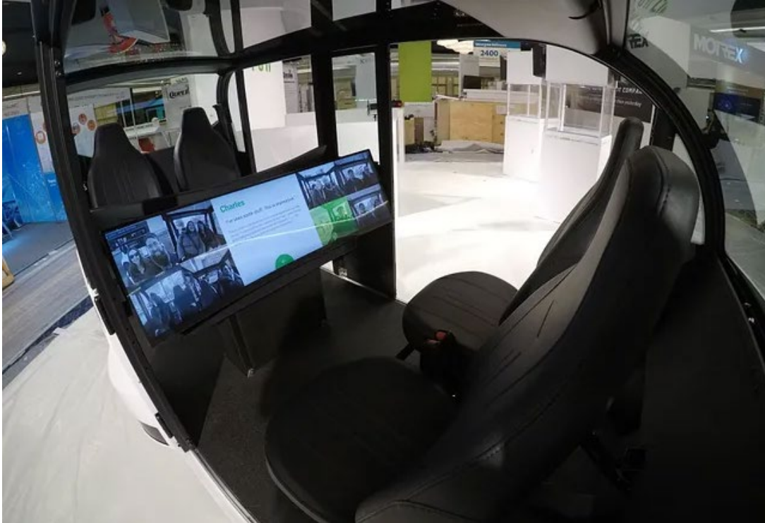
Figure 60. Interior concept of Myla 2.0 showing curved touchscreen and facing seat configuration (May Mobility, 2019).
