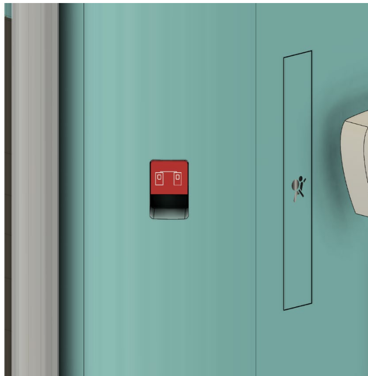
Figure 94. Airbag and Emergency Door Open Features
