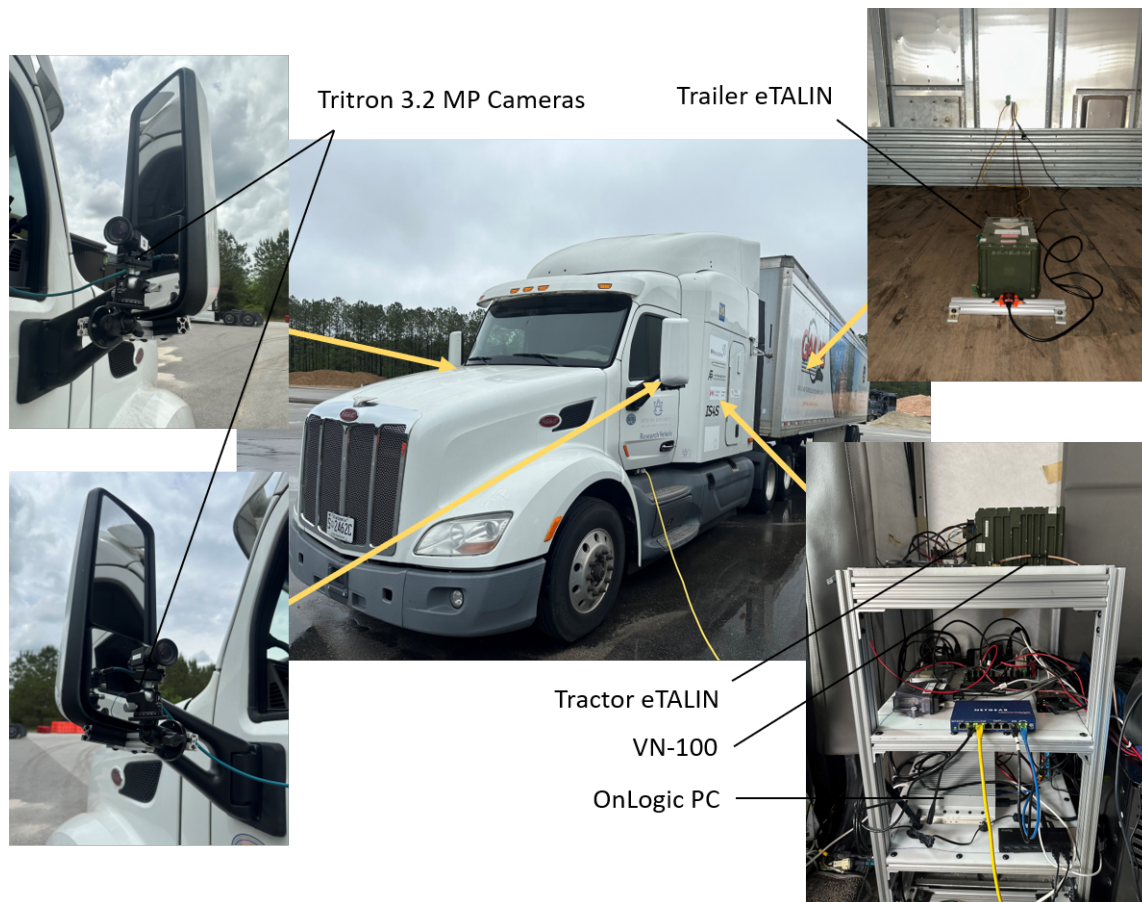
Figure 6.23: Test Vehicle Equipment Setup
