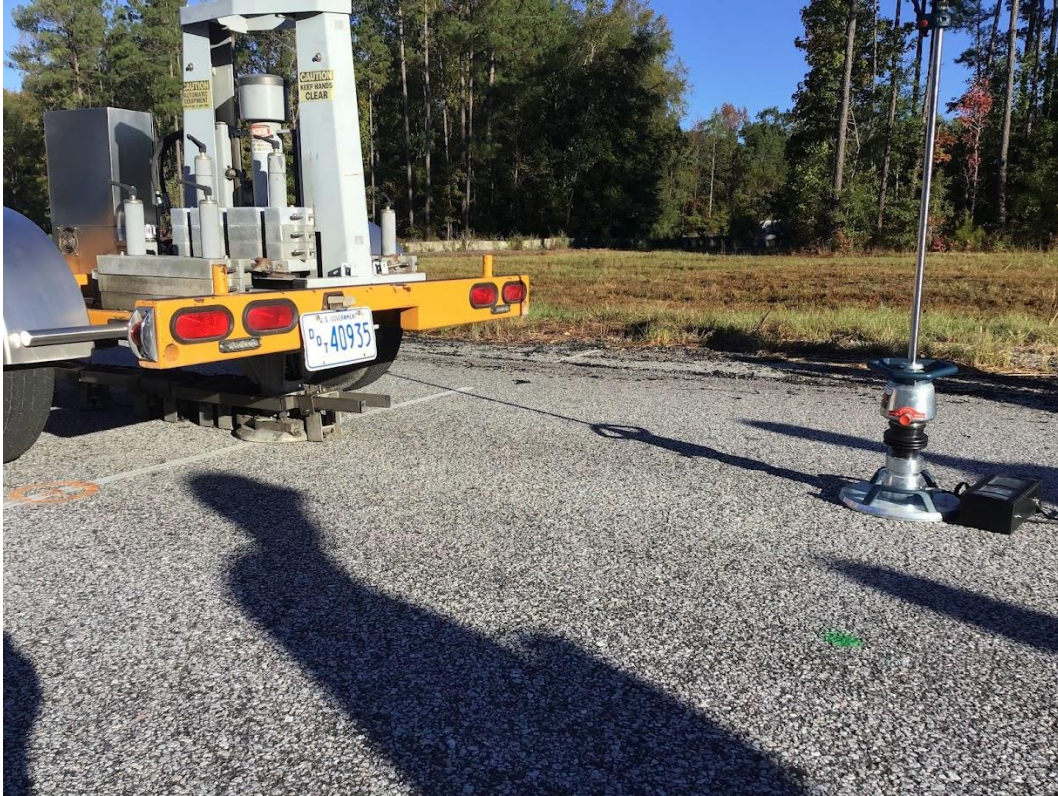
Figure 5.1: Test Track FWD and LWD Simultaneous Testing
