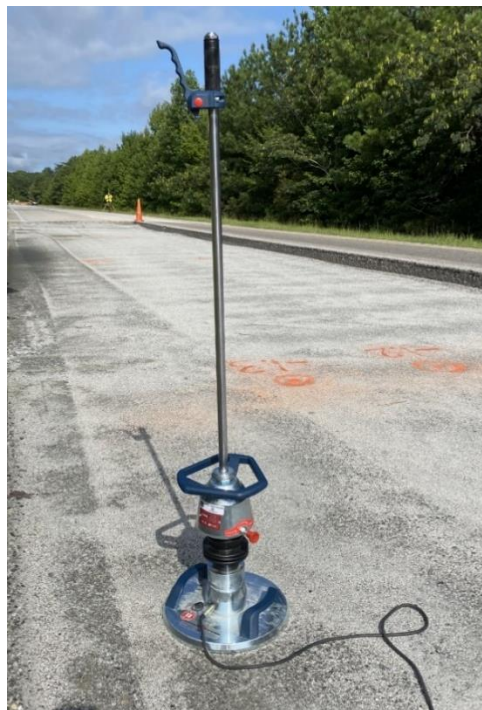
Figure 1.1: Zorn ZFG 3.1 on Aggregate Base at the NCAT Test Track
