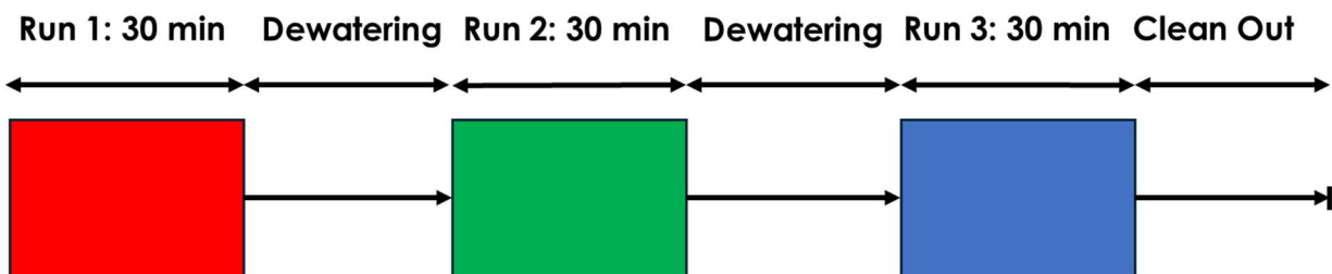
Figure 3.10: Silt Trap Testing Regime
